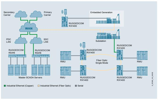
The RUGGEDCOM RX1400 can be used to connect low voltage substations and distributed generation plants reliably via public celullar networks.
