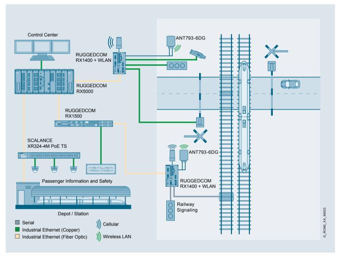
The RUGGEDCOM RX1400 provides redundant connection of end devices by fiber-optic and / or cellular networks for more reliability in case of network failure.
