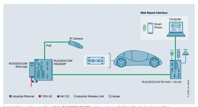
$Automated\ license\ plate\ recognition\ with\ the\ RUGGEDCOM\ RX1400\ running\ a\ custom\ application\ in\ the\ virtual\ environment\ from\ the\ RUGGEDCOM\ VPE1400$
