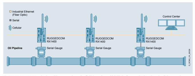
The RUGGEDCOM RX1400 makes it possible to remotely monitor field data using multiple kinds of communications through cellular networks, fiber-optics, or both in a redundant way.
