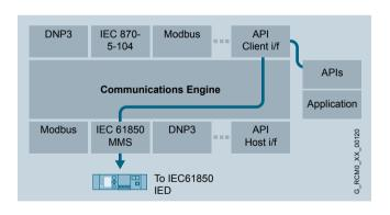
RUGGEDCOM ACE enables 3rd party applications to communicate with downstream IEDs via standard SCADA protocols, eliminating the need for developers to implement complex protocol stacks within their own applications.
